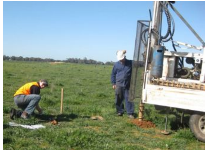
Figure 1 showing the Hydraulic Coring machine in operation and a student dissecting a soil core.
