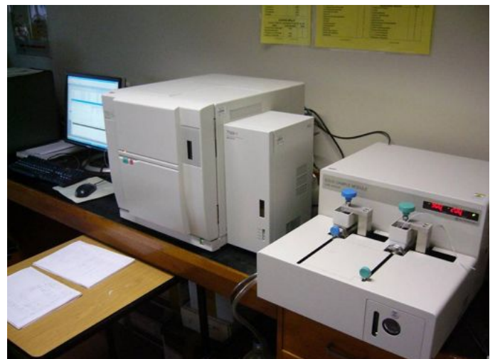
Figure 2 showing the Shimadzu Total Organic Carbon Analyser Solid Sample Module.
