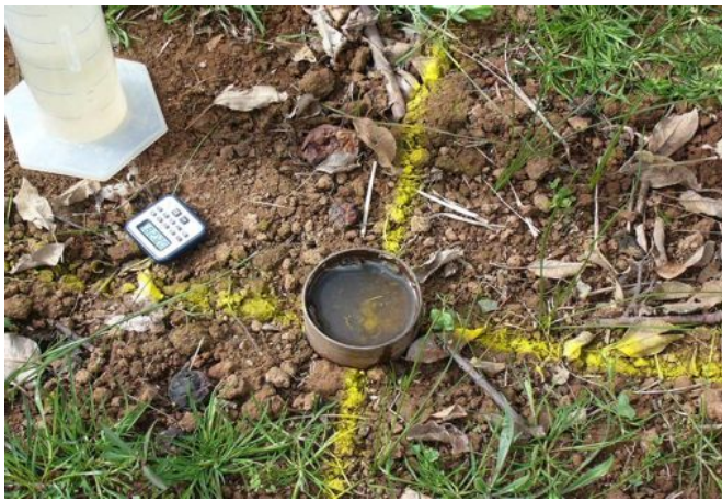
Figure 3 showing a soil infiltration test in progress.
