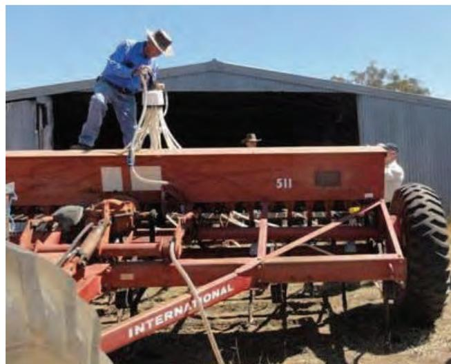
Fred Wheeler demonstrates the use of the BNS Easyflow for applying liquid nutrients.
